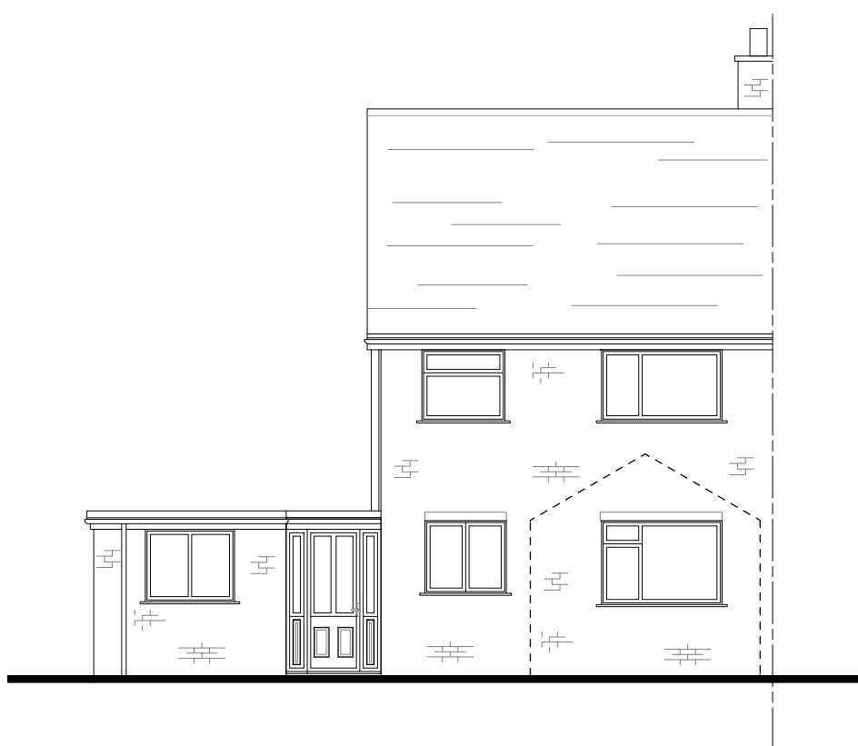
Existing Rear Elevation View C - 1:100
