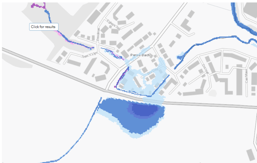
Figure 2: The area classified as Flood Zone 3 in the north east of the development. The screenshot has been taken from the NRW Development Advice Maps.
